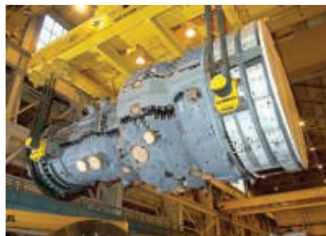
FIGURE 3. The modern, horizontally split gas turbine casing shown here is an example of a large and modern gas turbine. Today's advanced turbines are sophisticated and complex systems that allow for overall efficiencies above 50% (Photo used with permission from Siemens)
