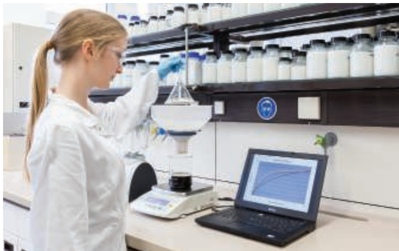
FIGURE 4. The rate at which pulp slurry is dewatered can be measured in drainage tests
