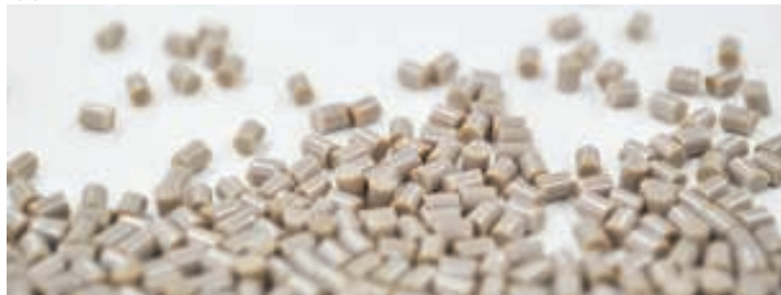
FIGURE 1. Victrex PEEK 90GL-30BLK EU was introduced to meet the current requirements of both U.S. and European regulatory authorities for direct-food-contact applications, while providing temperature performance and chemical and steam resistance, as well as wear resistance without lubrication
